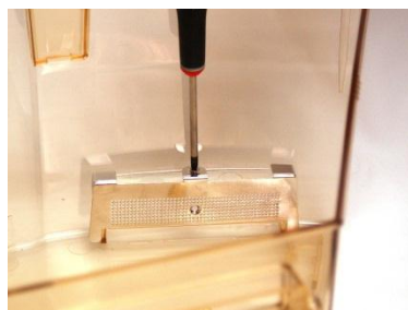
Figure 3: Securing metal screen
