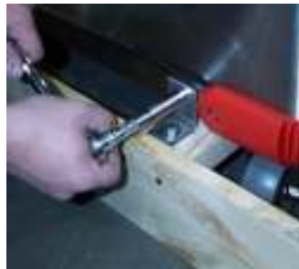
Remove all four (4) L-brackets holding rack to pallet with a 7/16" (or 11mm) wrench.
