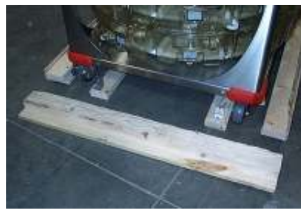
Knock off the 1 x 6 end piece of the pallet and unlock the two front casters.
