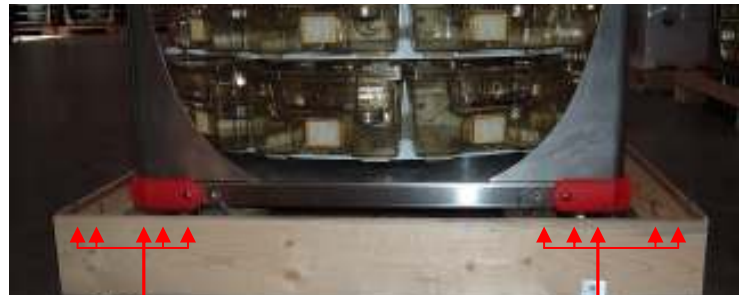
Remove ten (10) wood screws from the top of the pallet using a Phillips screwdriver.
